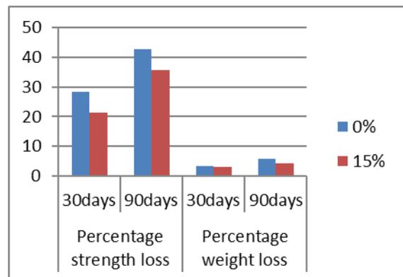
Fig 5. Influence of chloride attack on concrete
