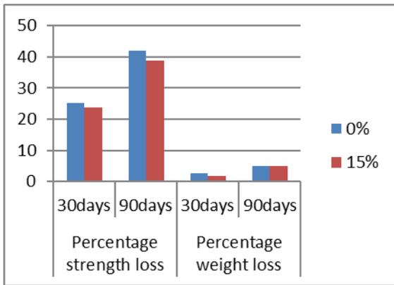
Fig 6. Influence of Sulphate attack on concrete
