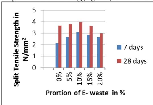
Fig 3. Effect of E-waste on split tensile strength
