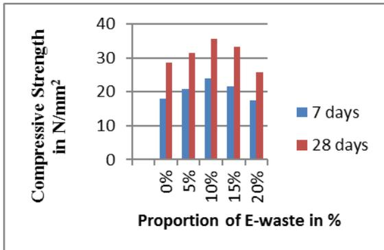
Fig 2. Effect of E-waste on compressive strength
