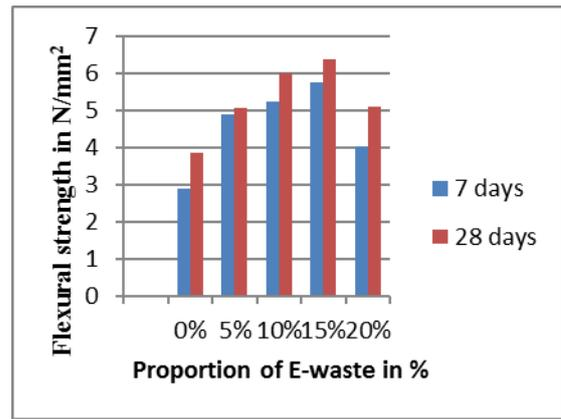
Fig 4. Effect of E-waste on flexural strength
