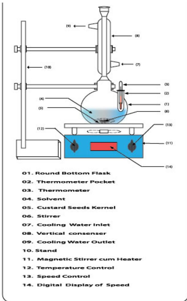
Fig 3. Schematic Diagram of experimental setup
