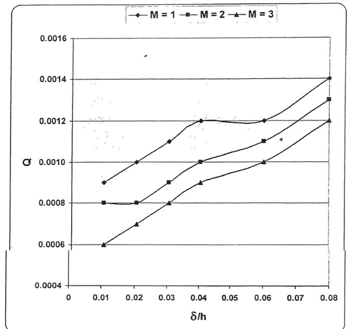
Graph – 1.1: Variation of flow rate with PPL thickness.
