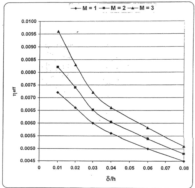
Graph – 1.4: Variation of effective viscosity with PPL thickness.
