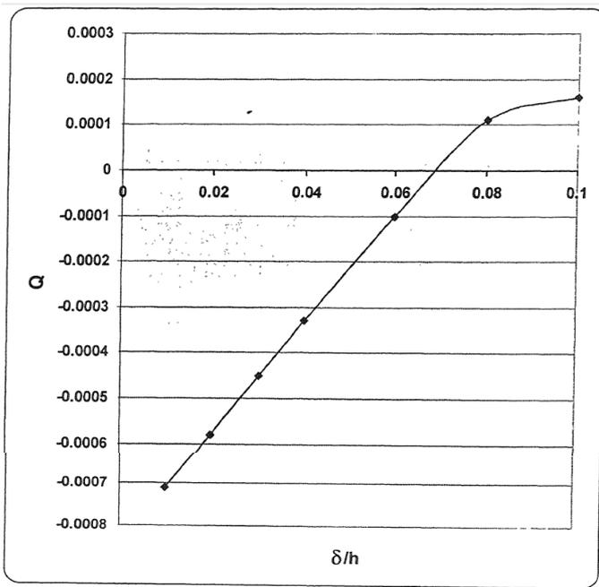
Graph – 1.2: Variation of flow rate with PPL thickness ( $m \rightarrow 0$ ).
