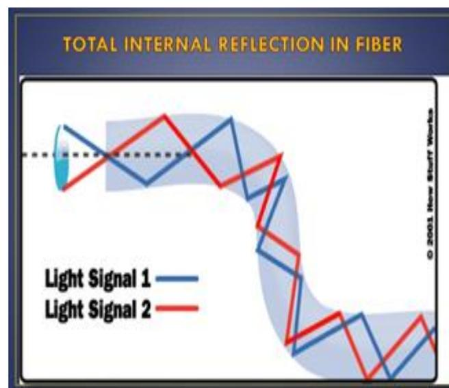
Fig 2.1 Total internal reflection in fibers
