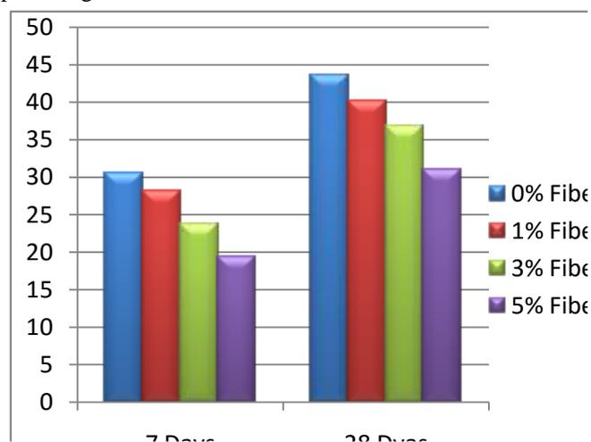
Fig 5.2 Compressive strength comparison of cubes of different percentage
