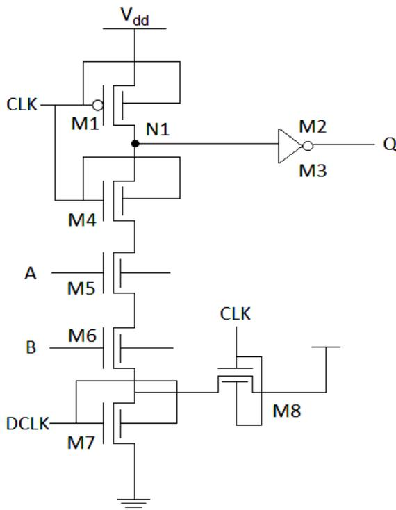
Fig 12: Proposed Technique AND Independent Gate using FinFET.
