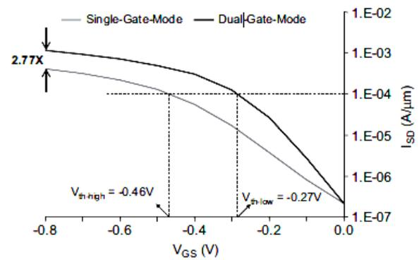
Fig. 8. Drain current characteristics of a single-fin P-type IG-FinFET. The source-to- drain voltage is 0.8V.  $T = 110$  IC.  $I_{off} = 216$ nA/mm.  $I_{on}$  (single-gate-mode) = 0.422 mA/um.  $I_{on}$  (dual-gate-mode) = 1.17mA/um. The threshold voltage is the gate-to- source voltage at which the drain current per fin height is  $10^{-4}$  A/um for  $|V_{DS}| = V_{DD}$ .
