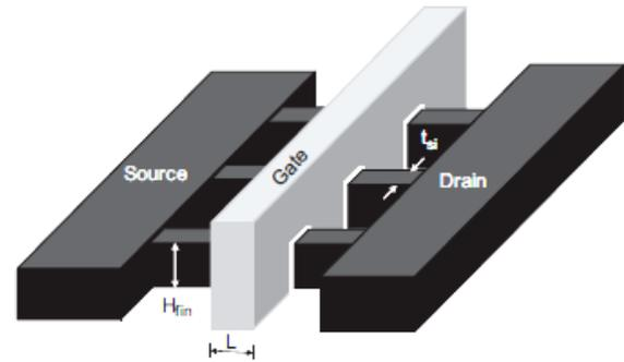
Fig 7. Three – FinFET.  $W_{total} = 3 \times (2 \times H_{fin} + t_{si})$ .
