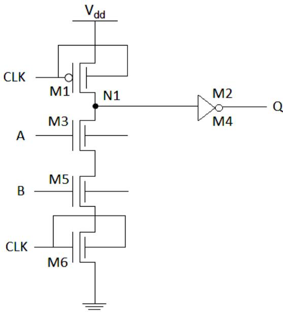
Fig. 10. Domino AND Independent Gate using FinFET.
