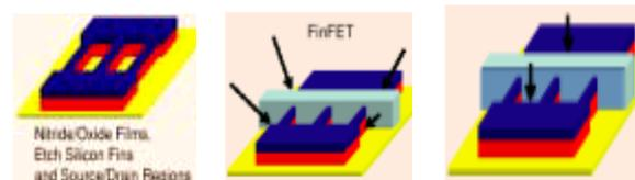
Fig 5. FinFET manufacturing process flow
