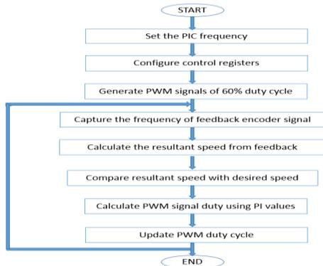
Fig. 8 Flowchart for the closed-loop control
