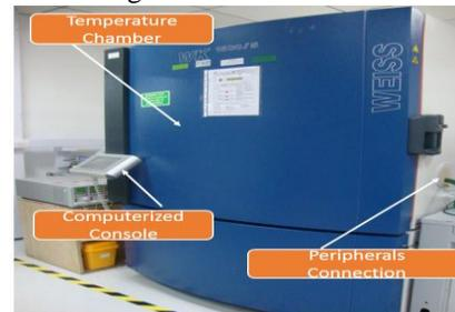
Fig. 10 HALT temperature test chamber
