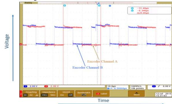
Fig. 15 Encoder feedback signal
