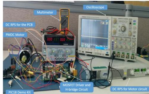
Fig. 9 Hardware setup
