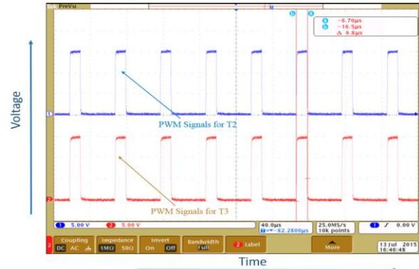
Fig. 14 PWM pulsed signals of low-side MOSFETs
