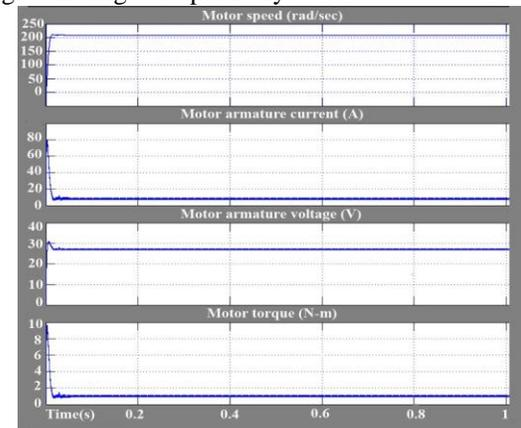
Fig. 6 Motor characteristics with PI controller
