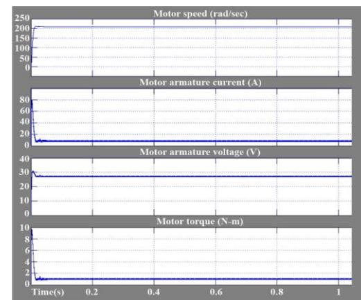
Fig. 7 Motor characteristics with PID controller
