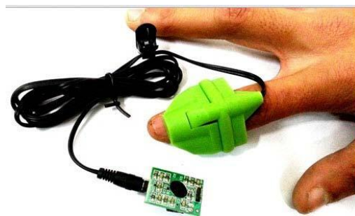
Figure.2. Heartbeat sensor with 8051 Microcontroller [3]
