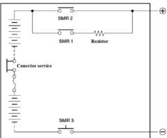
In the moment of disconnecting the system, SMR 2 and SMR 3 are switched off in this order and BMS checks if there relays where closed.
