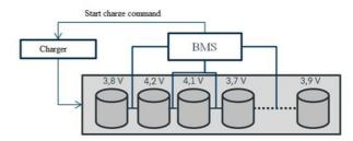
If the series connections, the first cell that reaches the minimum voltage cutting discharge determine battery capacity. Although other cells can still be discharged, the operation will be halted because the current will pass through the weakest cell and discharging it over the allowed limit, thus bringing the battery outside the range of its safe operation (SOA - Safe Operating Area). The same thing will happen when charging the battery.
