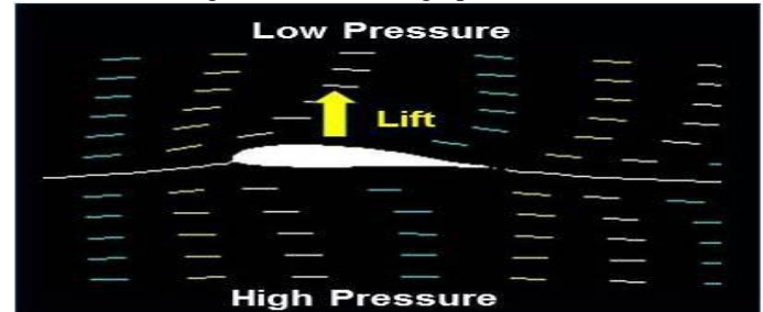
Fig.5: lift in an aerofoil
