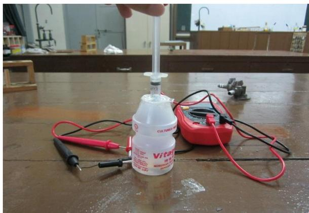
Figure 4 shows simulated breath prepared by diluting in static dilution bottle was injected into the breath-in apparatus which contained sensor by syringe.
