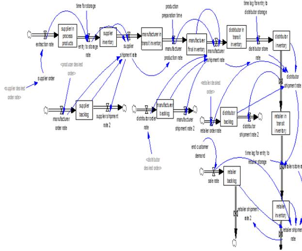
Fig2. Stock and flow diagram for order-shipment system of four-echelon supply chain
