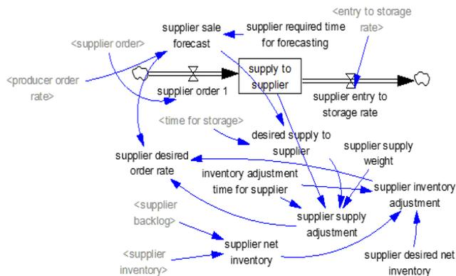
Fig3. Stock and flow diagram for desired order of supplier
