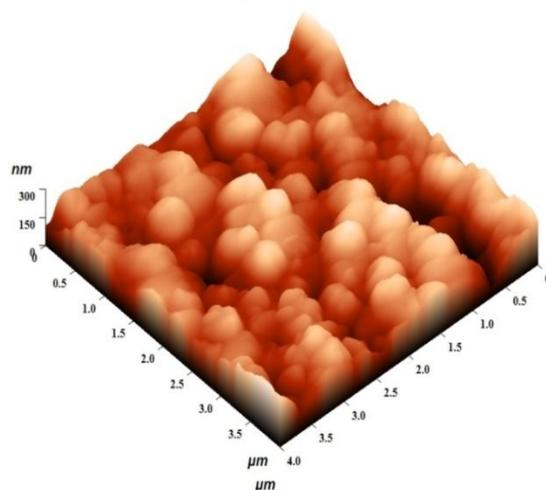
Fig. 4 AFM image of CdS thin films
