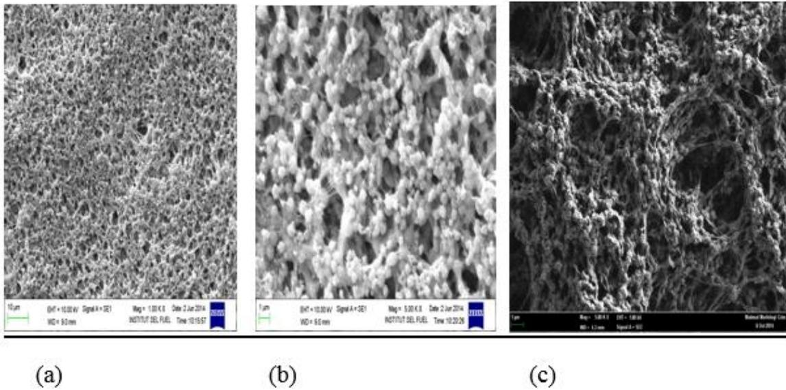
Figure 8. demonstrates the micrograph of the PVDF film, (a) and (b) SEM images of PVDF and (c) FESEM image of PVDF/ZnO.
