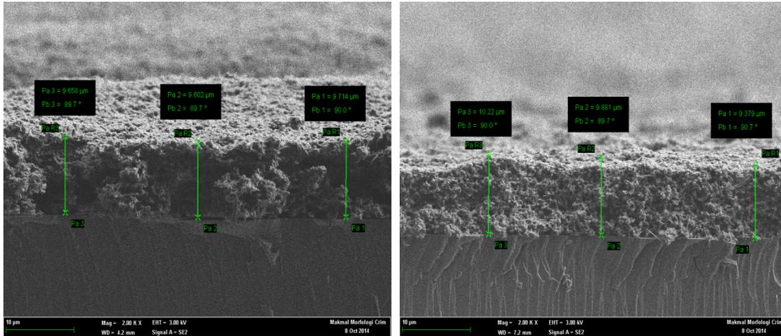
Figure 9 The FESEM cross section of the PVDF/ZnO film.
