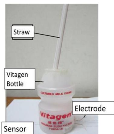
Figure 3 shows vitagen bottle with sensor adhered to the base inside (bottom).
