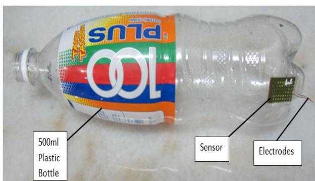
Figure 2 shows a 500ml plastic bottle with sensor inserted at the base (top)
