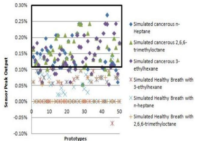
Figure 7 shows sensor peak output of SCENT when it was exposed to simulated lung cancer and healthy breath. Lung cancer breath induced greater resistance change when compared to healthy breath, as framed by the rectangular box.
