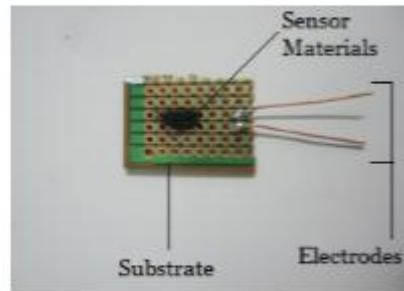
Figure 6 shows a fabricated sensor.
