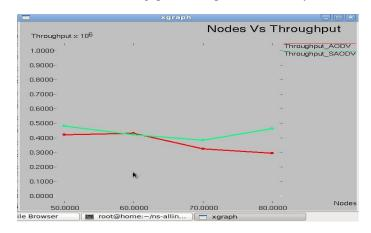
Figure 5 Throughput graph of AODV and SAODV
