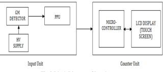
Fig 2 Block Diagram of Level gauge
