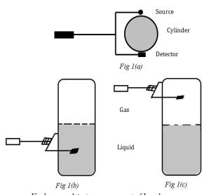
Fig 1 source detector arrangement of Level gauge
