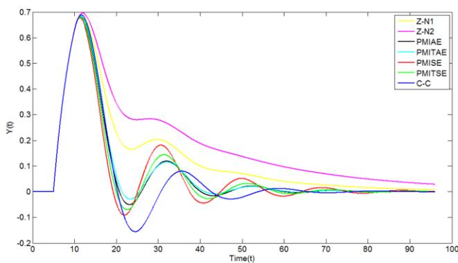
**Fig.6.** The comparison of tuning methods for the case study 2 ( $\tau_1 = 5, \theta = 5$ )
