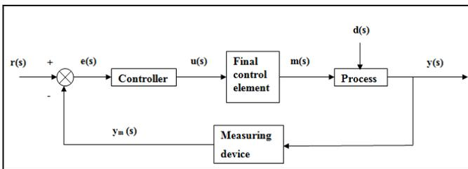
Fig. 1. Block diagram for conventional feedback control loop
