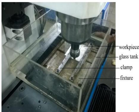
Fig.1. Submerged FSW setup
