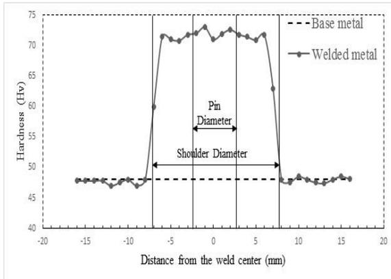
**Fig. 5. Vicker's hardness profile of base metal and the welded metal at optimum condition**
