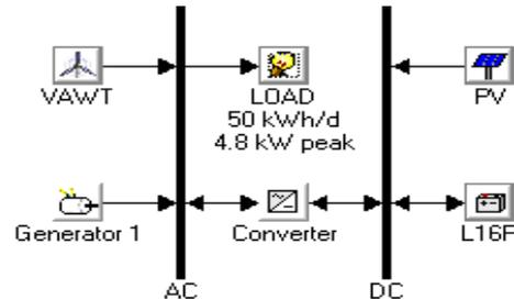
Fig.2. HOMER diagram for the hybrid system
