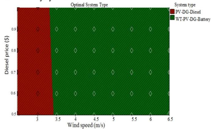
Fig. 8 Optimal system type over increase wind speed and fuel price for case 2 scenario 1
