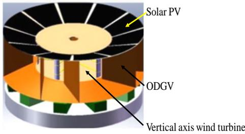
Fig.1. The Omni Direction Guide-Vane ODGV [10]
