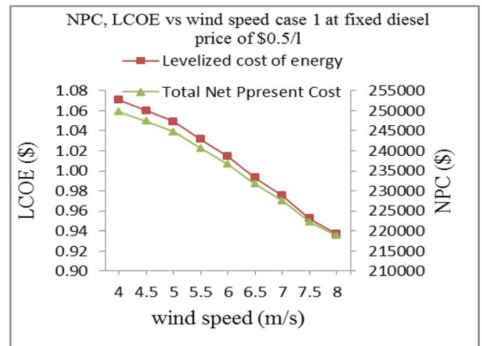
Fig. 9: Levelized cost of energy, NPC and wind speed
