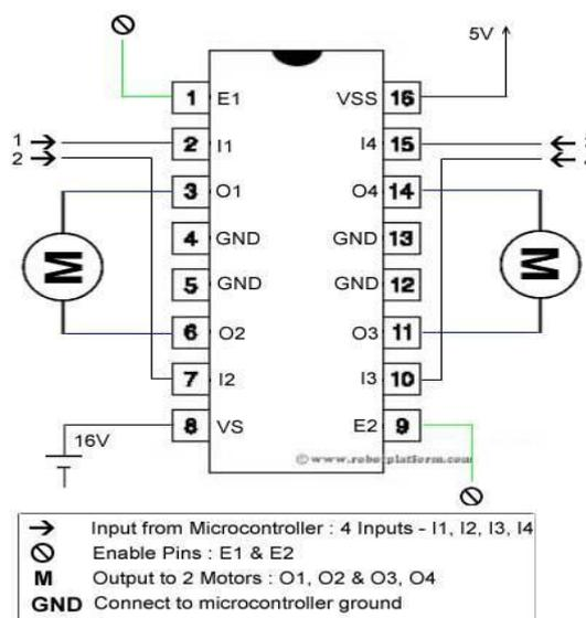
Fig 6. Pin Configuration of Motor Driver - L293D IC.
