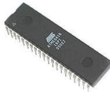
Fig 2. Atmega16 Microcontroller
