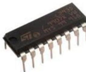
Fig 5. L293D Motor Driver
