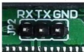
Fig 17.RXD, TXD, GND pin
