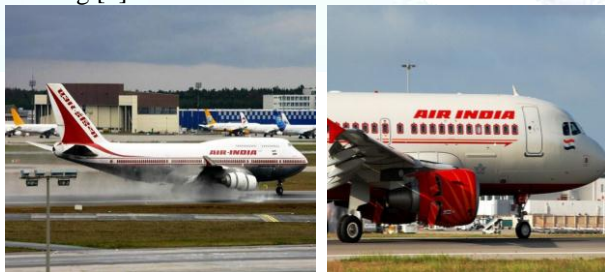
Fig.1 Thrust reversers deployed on turbofan of an Air India Boeing 747-400 landing at Indira Gandhi International Airport, New Delhi (left), Air India
