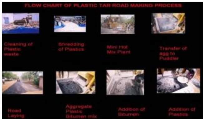
Figure 5: Plastic Tar making process with the help of Pictures
