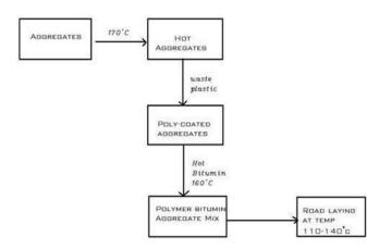
Figure 4: Flow Chart for Process of Mixing and Placing
