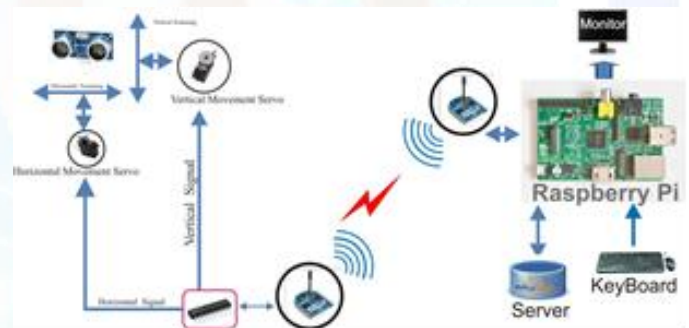
Fig.-1: System over View
