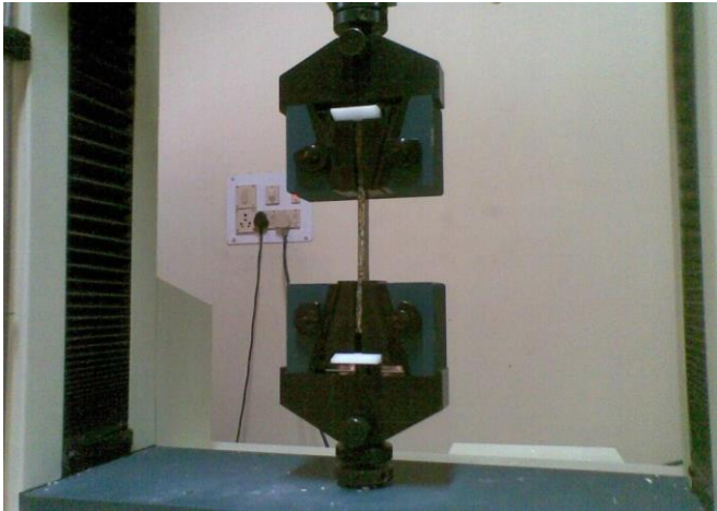
Figure 3.4 (b) UTM machine sample loaded for tensile testing
