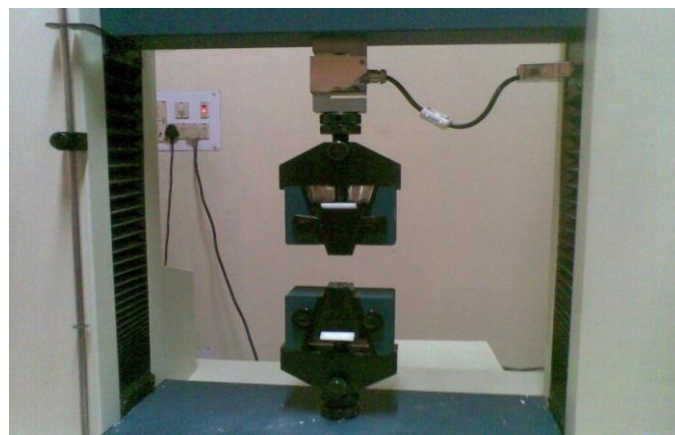
Figure-3.4 (a) UTM machine sample unloaded for tensile testing
