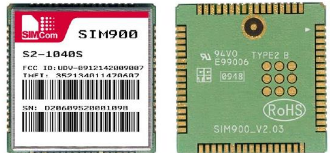
Fig 1.2 GPRS Module (SIM900)
