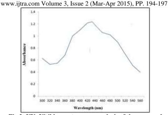
Fig 2: UV- Visible spectroscopy analysis of the prepared AgNPs. Presence of clear peak at about 420 nm confirms the synthesis.
