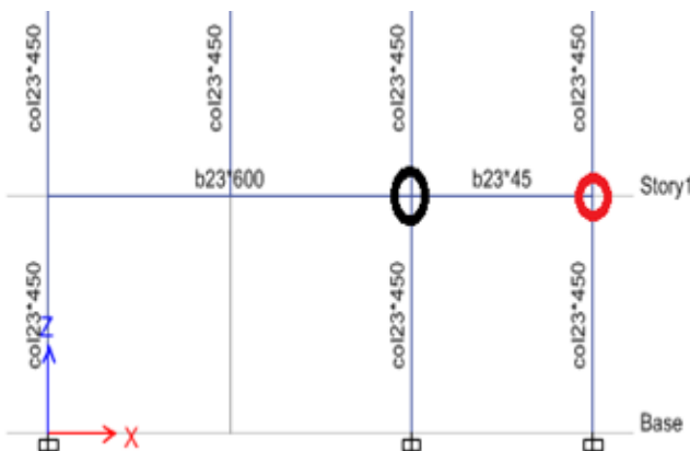
Figure 14. Columns directly Exceeding the CP level
