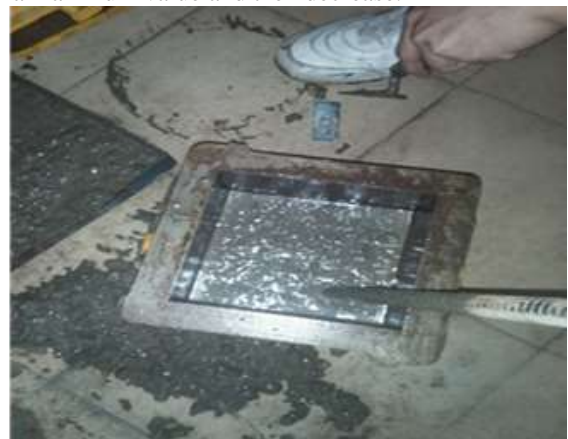
Figure 8: Compaction of cube with tamping rod during casting
