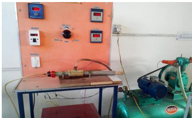
Fig. 3.3 Temperature measurement of Vortex tube
