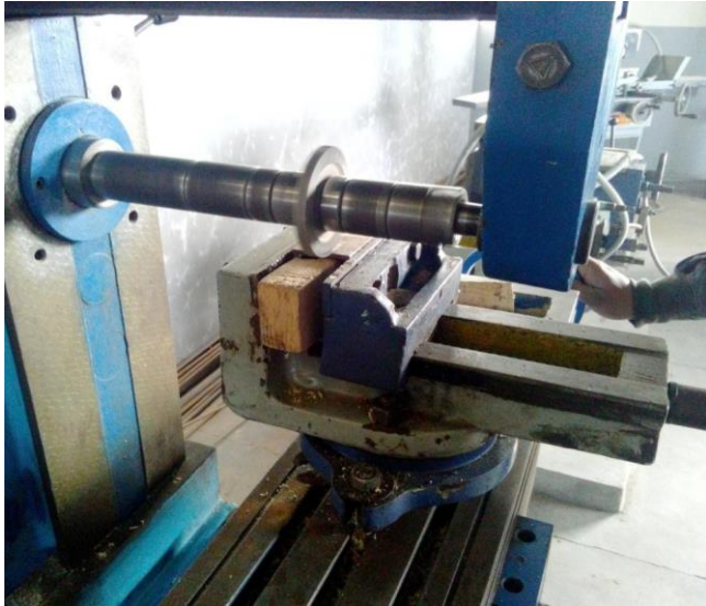
Fig. 4.4 Milling of mild steel specimen without coolant
