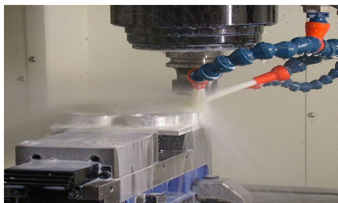
Fig. 1.1 Thin-wall milling of Aluminium using water - based cutting fluid on the milling cutter
