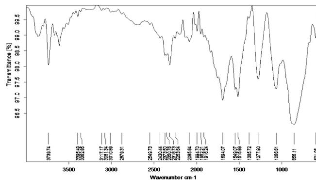
Figure 13 FTIR Spectrum of Pure KDP Crystal
