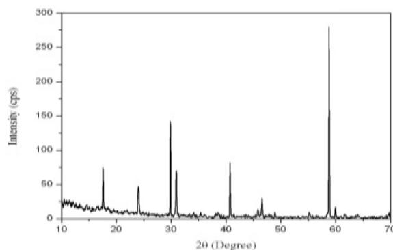
Figure 7 XRD Pattern of grown L-Methionine doped with KDP single crystals
