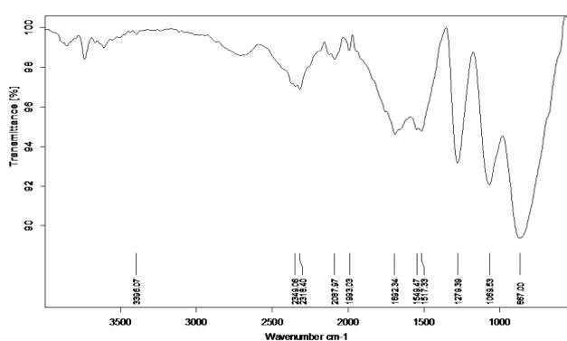
Figure 20 FTIR Spectrum of L-glutamic acid (0.6 g) doped KDP Crystals
