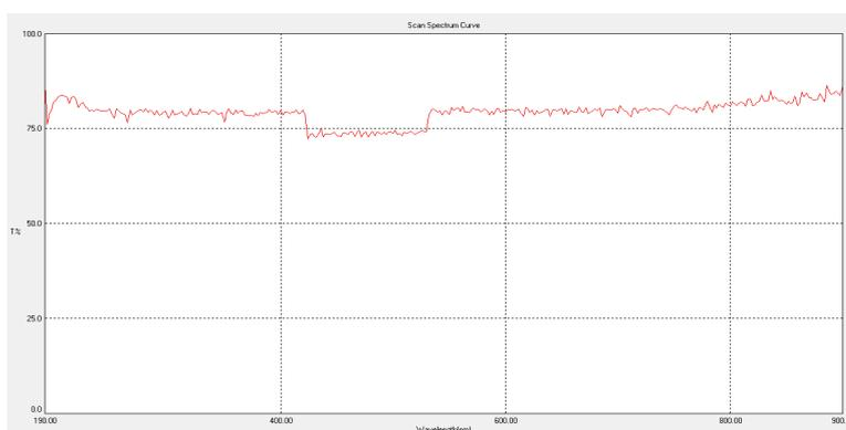
Figure 12 UV Transmittance spectrum of L-Glutamic acid (0.2g) doped KDP crystals
