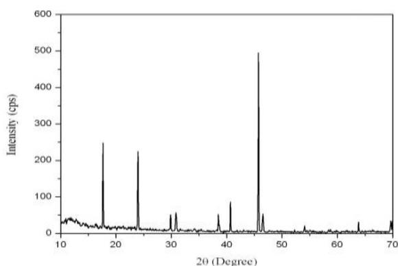
Figure 5 XRD Pattern of as grown pure KDP crystals
