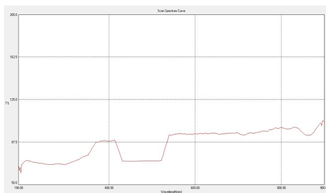
**Figure 9 UV Transmittance spectrum of Pure KDP crystals**
