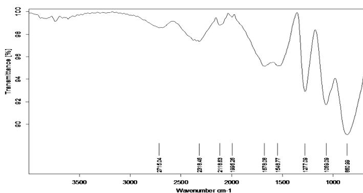
Figure 17 FTIR Spectrum of L-Methionine (0.4g) doped KDP Crystals
