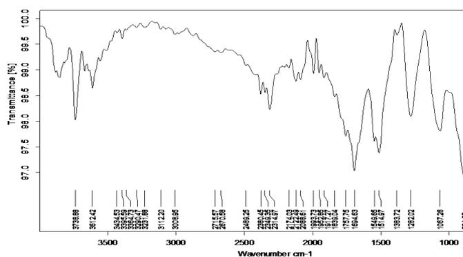
Figure 16 FTIR Spectrum of L-Methionine (0.6g) doped KDP Crystals
