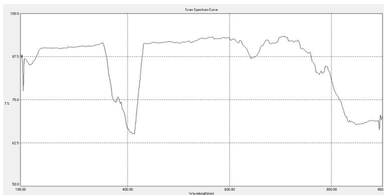
Figure 11 UV Transmittance spectrum of L-Methionine (0.2 g ) doped KDP crystals
