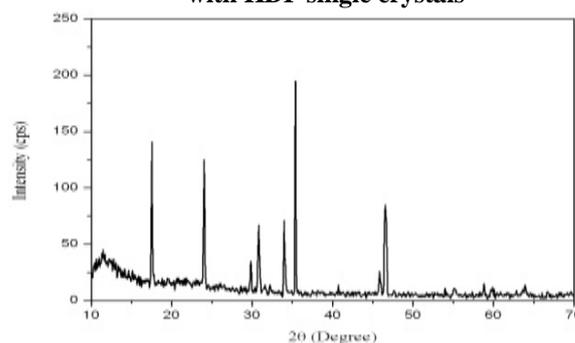
Figure 8 XRD Pattern of grown L-glutamic acid doped with KDP single crystals
