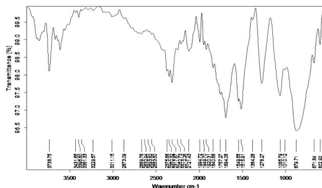
Figure 15 FTIR Spectrum of L-Methionine (0.2g) doped KDP Crystals
