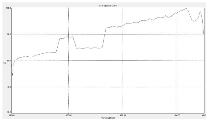
**Figure 10 UV Transmittance spectrum of L-Phenylalaine (0.2g) doped KDP crystals**
