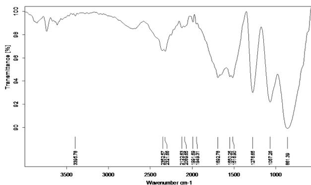
Figure 19 FTIR Spectrum of L-glutamic acid (0.4 g) doped KDP Crystals
