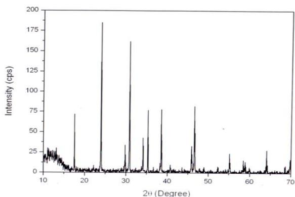
Figure 6 XRD Pattern of grown L-phenylalanine with doped KDP Crystals
