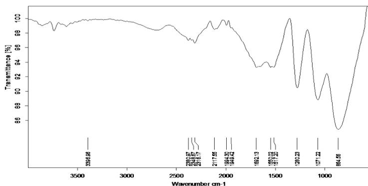
Figure 18 FTIR Spectrum of L-glutamic acid (0.2 g) doped KDP Crystals
