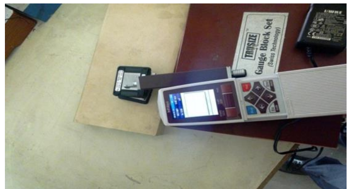
Fig. 4.2 Measurement of surface roughness
