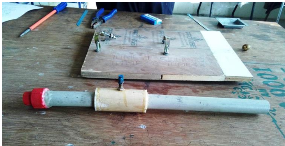
Fig 3.1 Fabrication of vortex tube
