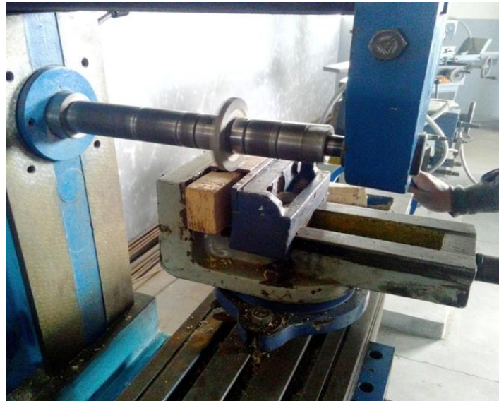
Fig. 4.4 Milling of mild steel specimen without coolant
