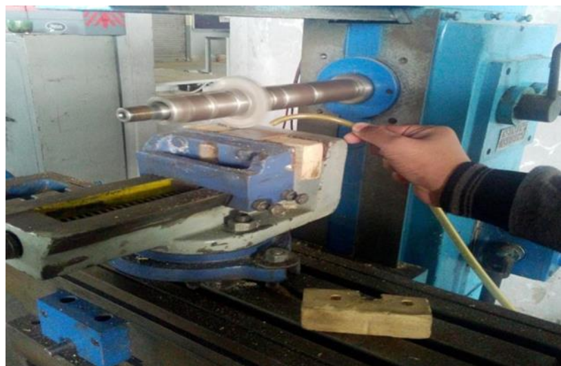
Fig. 4.5 Milling of mild steel specimen with vortex tube cooling
