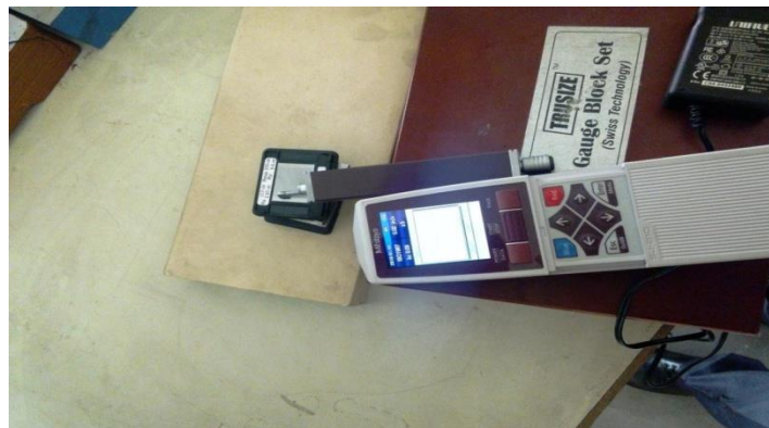
Fig. 4.2 Measurement of surface roughness
