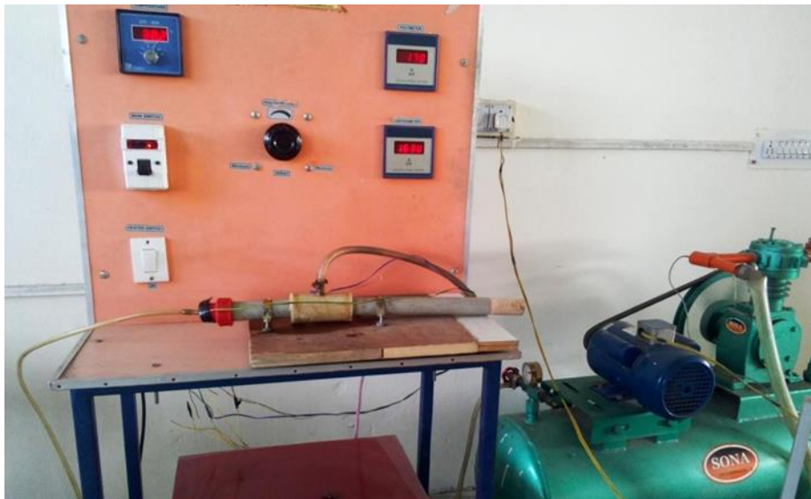
Fig. 3.3 Temperature measurement of Vortex tube
