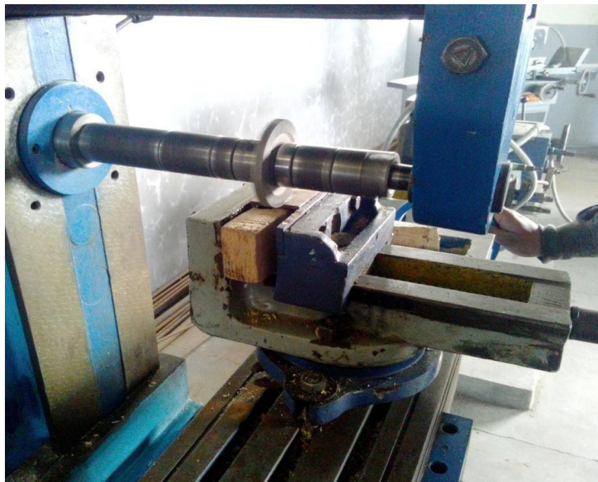
Fig. 4.4 Milling of mild steel specimen without coolant
