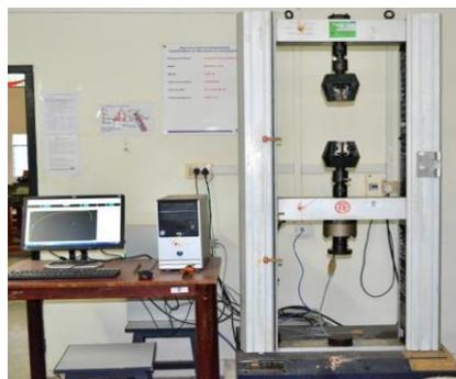
Figure 4.8 Universal Testing Machine used for the tensile experiment
