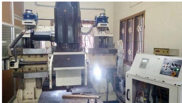
Figure 4.4 Welding machines utilized for the fabrication of the joints
