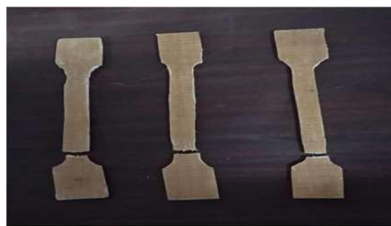
Fig. 5.1(b) Specimen after Fracture
