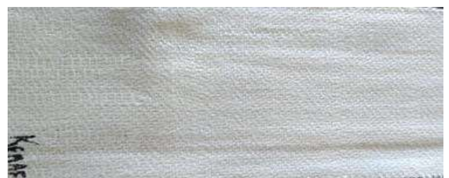
Fig.3:2 Kenaf Mat (00 / 900 Orientation)
