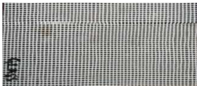
Fig. 3.3 E-Glass Mat (00 / 90° Orientation)
