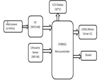
Fig. Block diagram of overall system
