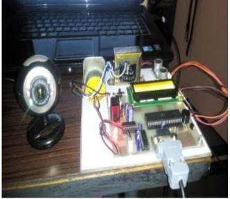
Fig. Hardware input When the power supply is provided to the hardware the LCD, DC Motor and buzzer are powered on.
