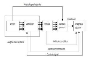
Fig. Controller based drowsiness detection system
