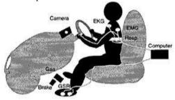
Fig. Sensors measuring the physical response
