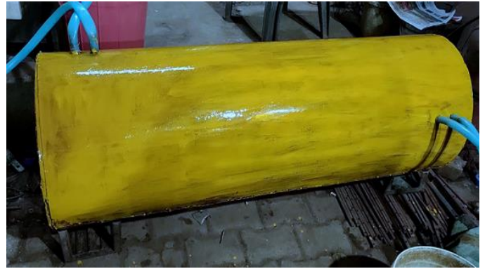
Shell and tube heat exchanger with 9 baffle plates
