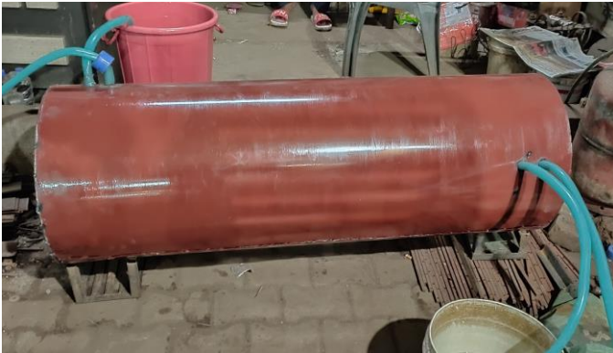
Shell and tube heat exchanger with 7 baffle plates
