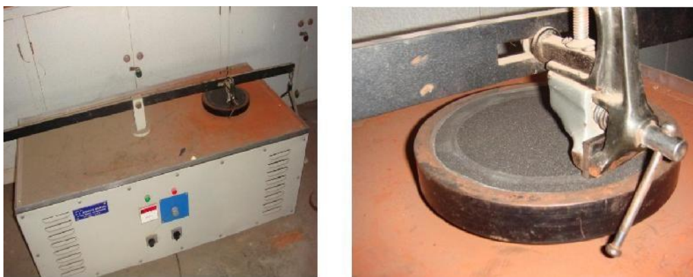
Fig. 2 Pin on disc machine for abrasive wear testing
