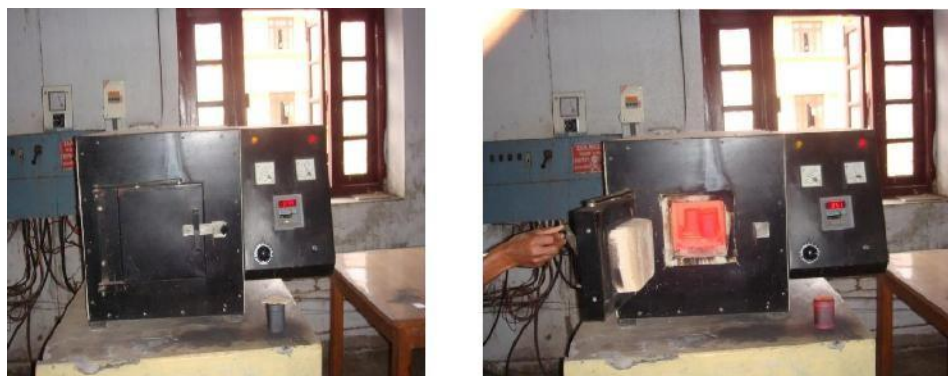
Fig. 1 Muffle furnace for carburization of mild steel samples
