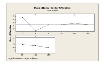
Fig 4.1: S/N Ratio graph for each parameter at different levels
