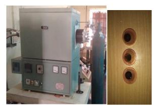
Fig. 3.4: Horizontal Tubular Furnace Fig. 3.5: Samples after sintering
