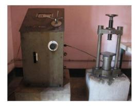
Fig 3.3: Cold Uniaxial Pressing Machine
