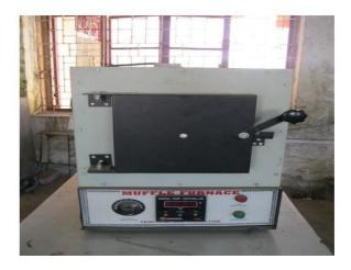
Fig. 3.7: Closed Muffle Furnace
