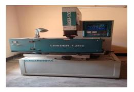
Fig 3.8: Electro discharge machine
