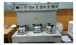
Fig 3.1: Ball Planetary Mill
