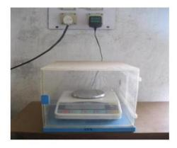
Fig 3.2: Electronic weighing machine
