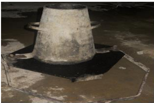
Fig -2: Slump Cone Apparatus
