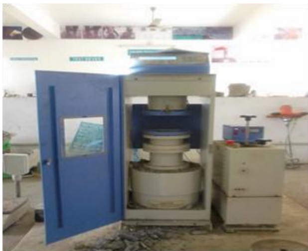
Fig -7: Compression testing machine of 2000KN
