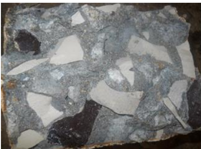
Fig -8: Concrete Specimens after testing
