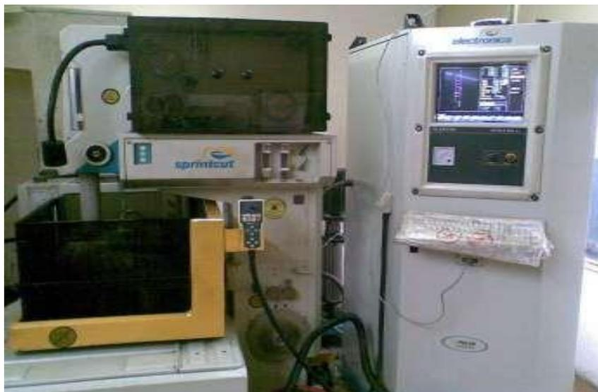
Figure 2.3: Experimental set-up of wire cut EDM [Courtesy NSIC, Aligarh (India)]
