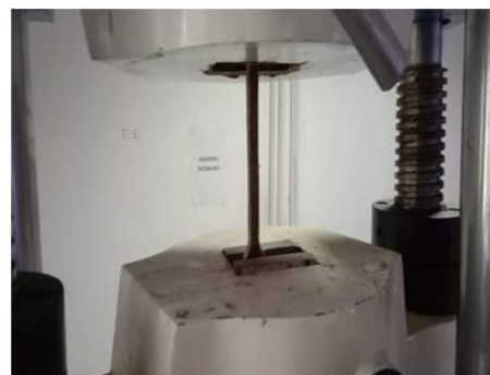
Fig-9(b): Specimen fixed hinged job
