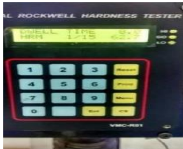
Fig-14(b): Hardness Test Reading on M scale
