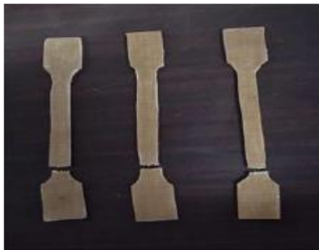
Fig-10(b) : Tensile Specimen after Fracture
