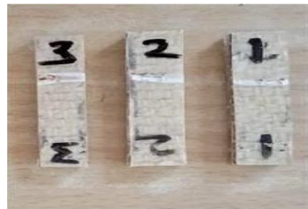
Fig-13(a): Impact Specimen Before Fracture
