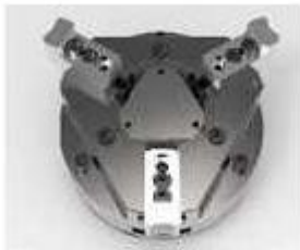
Fig 3.3 Ideal CNC 3 jaw chuck fixture
