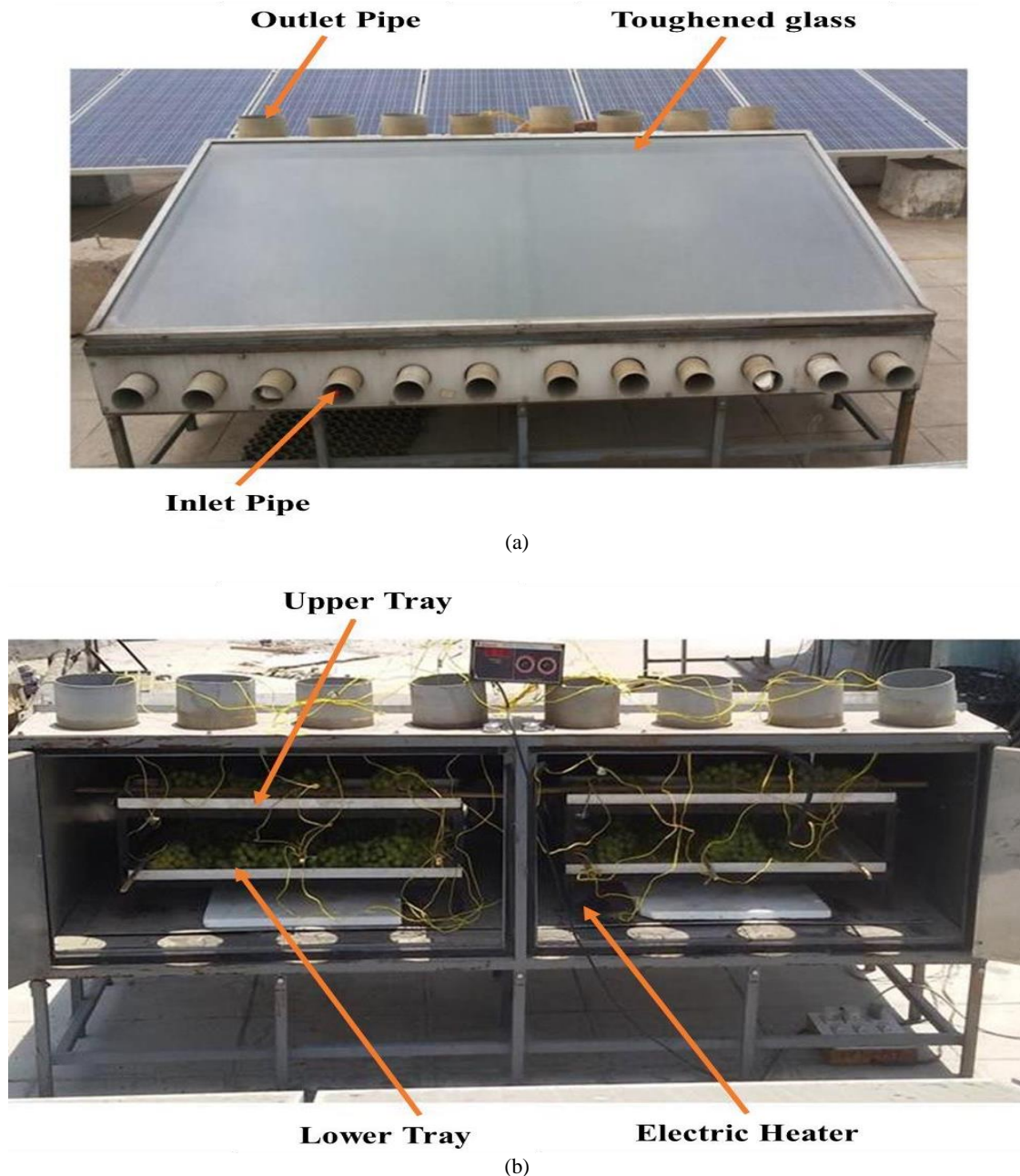
Figure 3.2 (a) Photographs of front and (b) side view of the solar dryer test setup.
