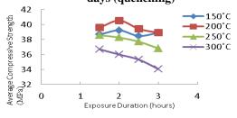
Fig. II Average cube compressive strength of NVC after 28 days (quenching)
