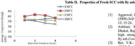
Fig I Average cube compressive strength of SCC after 28 days (quenching)
