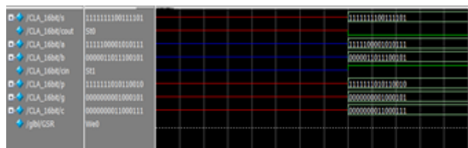
Figure 4: Addition using 16 Bit Carry Look-Ahead adder
