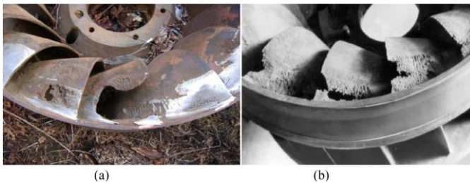
Figure 3. Cavitations Damage to Francis Turbines (a) [18] and (b).[19].
