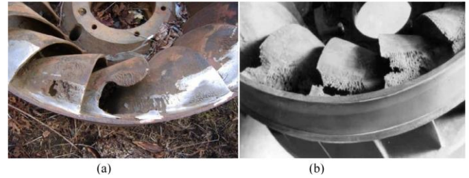
Fig. 4. Turbines (a) Misalignment detection and (b) Breakage of wicket gate linkage.
