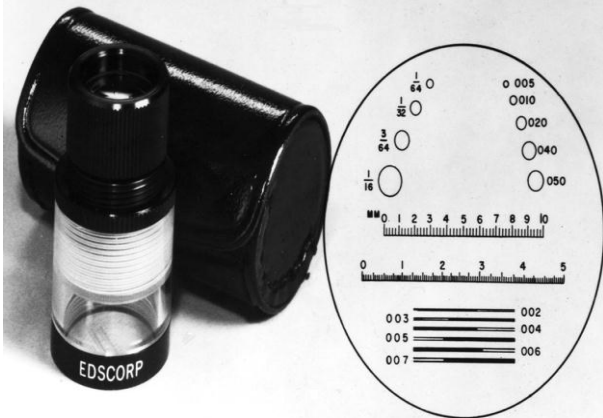
Fig. 3.1.1—Comparator for measuring crack thicknesses
