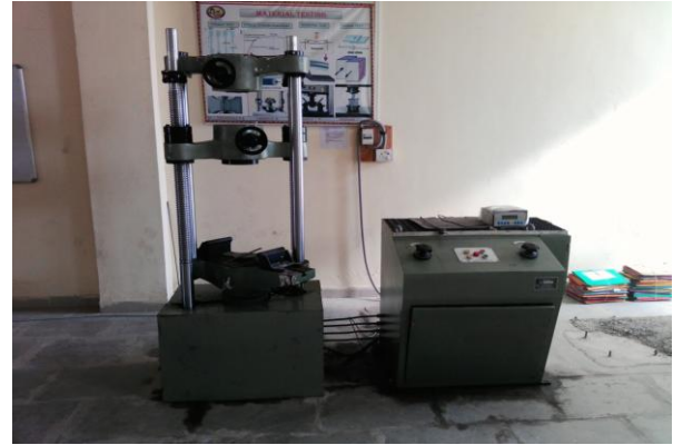
fig: Pull out Test set up
