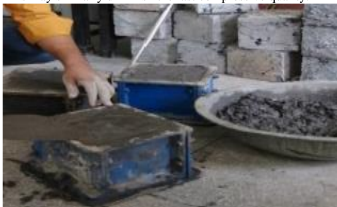
Fig. 8 Casting of Cubes
