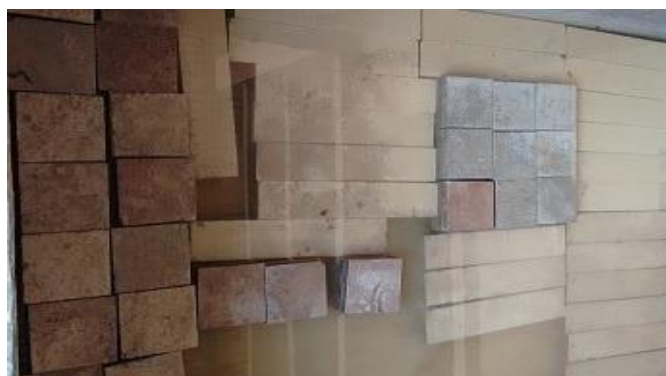
Fig. 9 curing of beams and cubes
