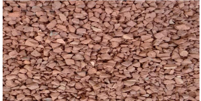
Fig. 2 Over burn brick aggregate used
