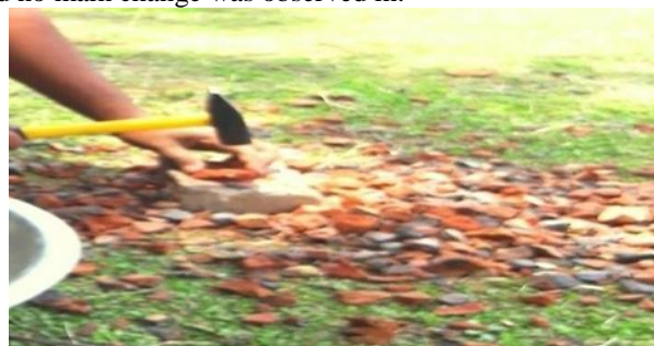
Fig. 3 Sample preparation of over burn brick aggregate
