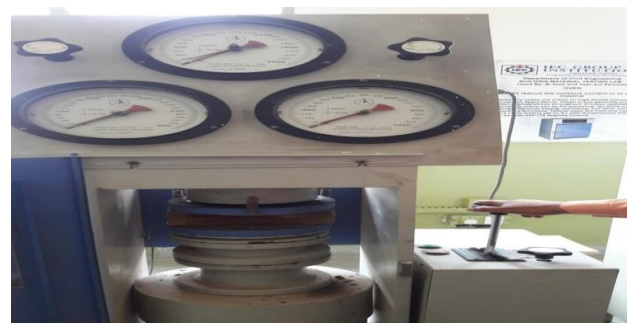
Fig. 5 Compressive strength test of over burn brick
