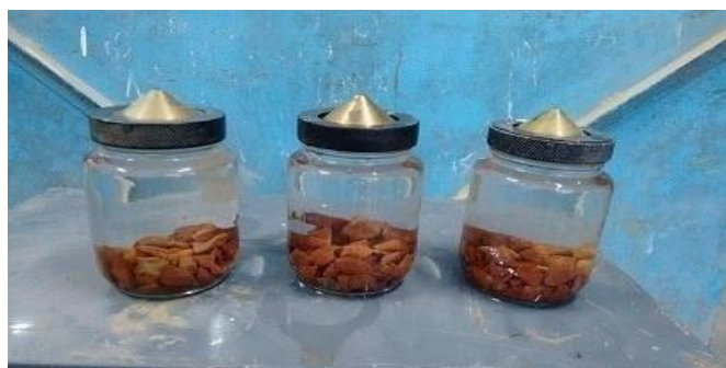
Fig. 6 Specific gravity test of over burn brick aggregate
